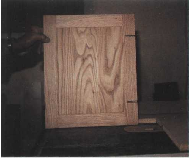
8 The back of the door shows the dados cut to receive the hinges.
