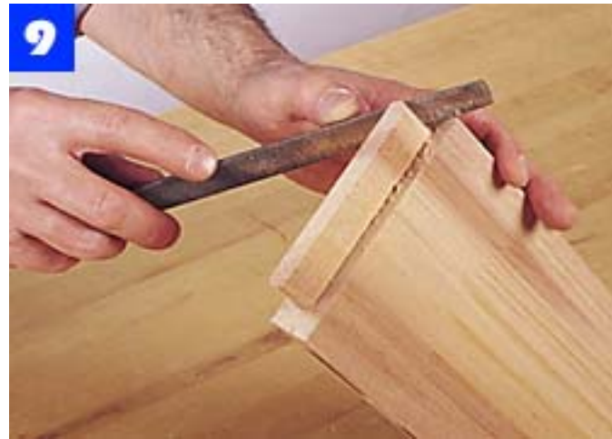
Round off a tenon with a rasp. The tenon's radius matches the radius left by the spiral up-cutting bit used to cut the mortise.
