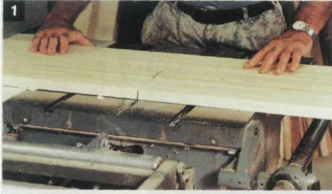
1 Cutting glued-up ends to finish dimensions
