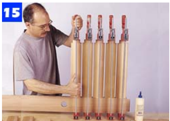
Multiple subassemblies are made in assembling the tabletop. First, slats are joined to the center rail.
