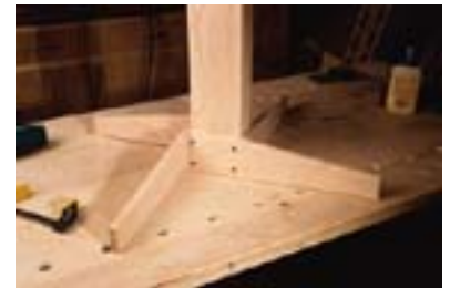
The feet are attached to the column with flat-head screws. Watch the screw alignment or you'll drill into another screw.
