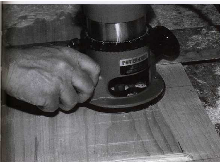
Use your square to mill the stopped dadoes that will receive the top, bottom and web frames.
