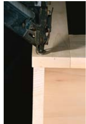
I'm not perfect, and neither are you. If your face frame is exactly the width of your case, it's going to be difficult to fasten it square. Make life easier by ripping your stiles \frac{1}{16} " oversize in width. After you nail and glue the face frame to the case, use a flush-trimming bit in your router to trim the face frame flush with the side of the cabinet's case.
