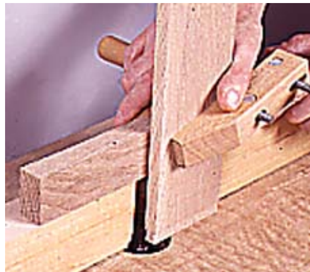
13--Rout slots in the drawer face for the drawer sides with a dovetail bit. Use a square U-shaped jig to guide the router.
