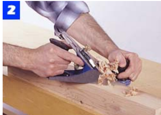
Clamp a table leg to a benchtop and remove saw marks with a hand plane. To make a smooth cut, push the plane at an angle.
