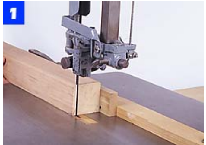
Rip the table leg stock out of a cedar 4 x 4. Clamp a temporary rip fence to the band saw table to do this.
