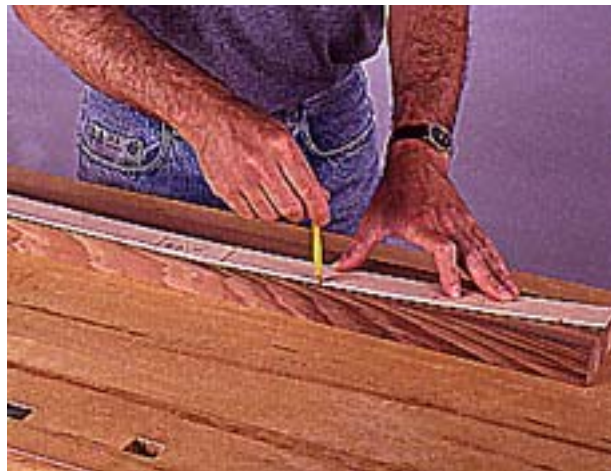
12 The first step in building each chair is to make a template for the rear leg, and trace it on the leg blanks.
