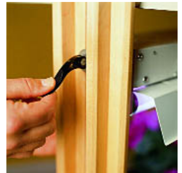
Light intensity is controlled by varying the lamp height. A well-adjusted cam clamp makes locking quick and simple.
