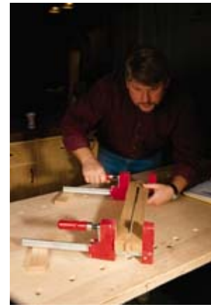
To form the post, the rough piece is ripped into three pieces, the center piece is cut to form two small blocks, and then the whole thing is glued back together.
