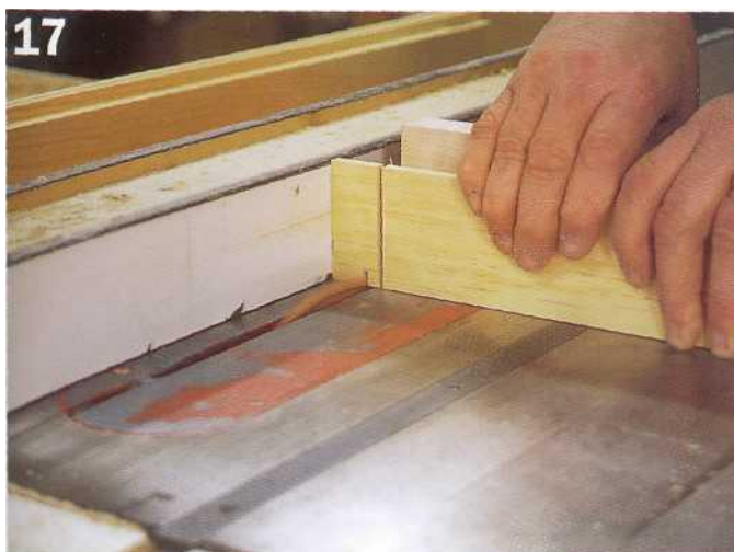
step 17 Raise the blade to 3/8" and make the outer edge cut.
