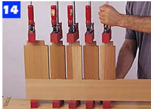
The first stage in assembling a benchtop is to glue and clamp slats to one stile. Use one clamp in the center of each slat.
