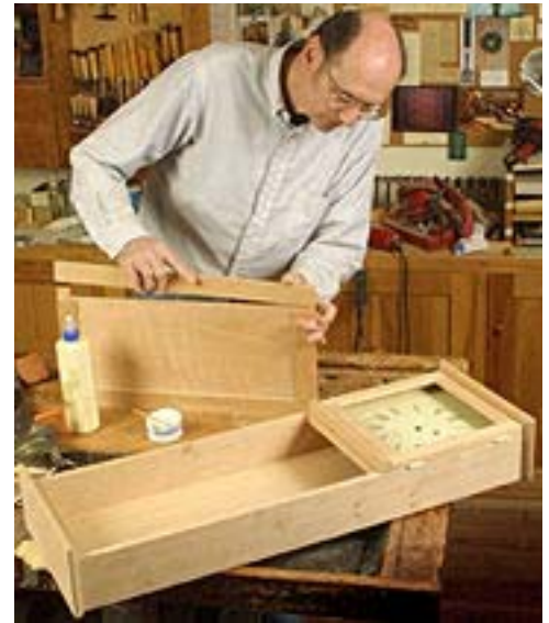
Before applying glue, carefully dry-fit the doors and see that they fit the case.
