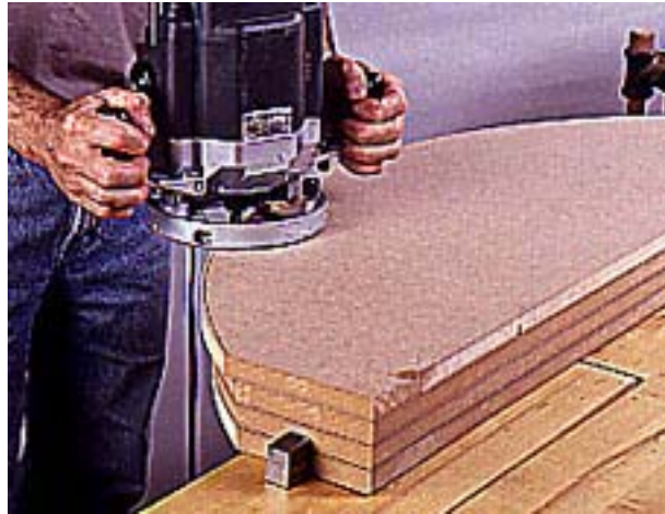
1 Make the bending form template with a plunge router on a trammel arm. Cut an arc in a sheet of MDF.
