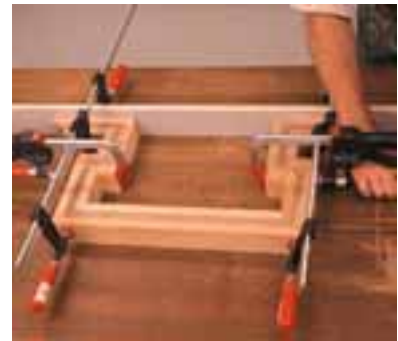
This is where your parts start to look like something. Joining the three assemblies creates the Greek key at the bottom of the base.
