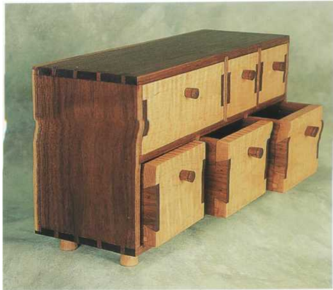
Partially open drawers reveal the fat dovetails.
