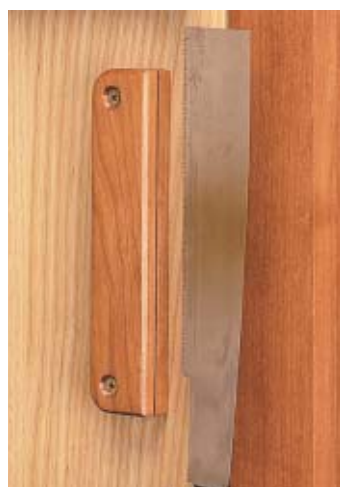
Hand saw. A kerf can be used to protect the teeth of a hand saw. To support the saw, I added a simple base, see main photo.
