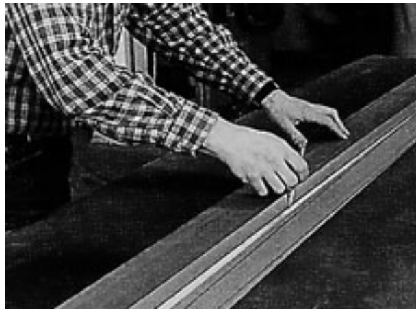
1 Rip and crosscut the post blanks, and use a long straightedge to mark the taper. Also mark the mortise positions.
