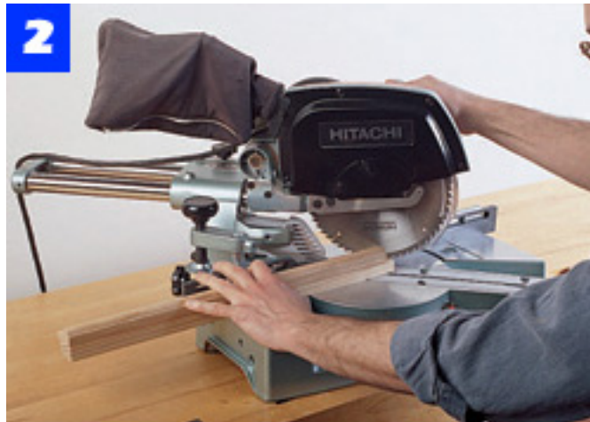
Use a miter saw to make the 45^\circ cuts at both ends of each piece. Make sure opposite pieces are the same length.
