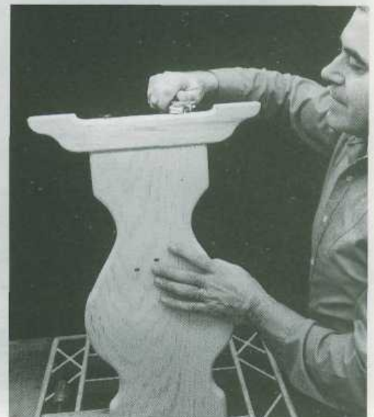
Fig. 11-4. Use lag screws to join shaped pedestal and base sections, as well as the top section to the pedestal. Use washers under screw heads.
