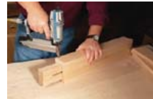
As you glue up the column, use the post to check the spacing. The post should slip easily into the sleeved column. You want the post to move easily, but don't make it too loose or you'll make the stand wobbly.
