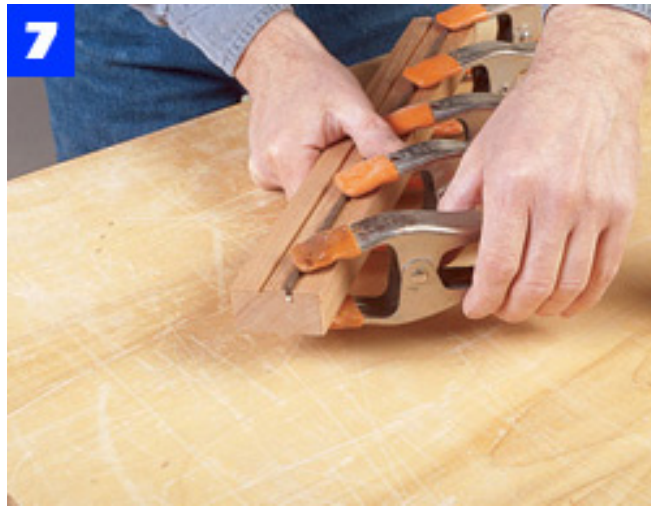
Frame 3 has two inlaid strips. Cut the slots on a table saw. Glue the strips in place and rout a chamfer on the edges.
