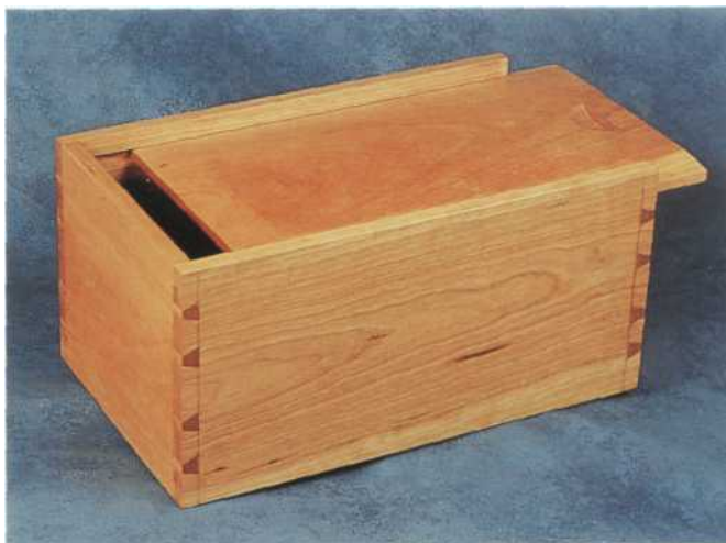
The open top of the candlebox lid reveals the grooves the lid rides in.
