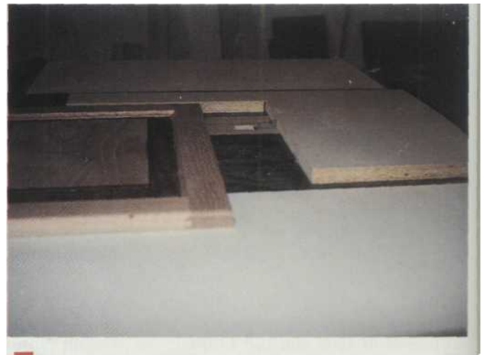
7 The edge view of the door shows the through tenon and groove used to assemble the stiles and rails.
