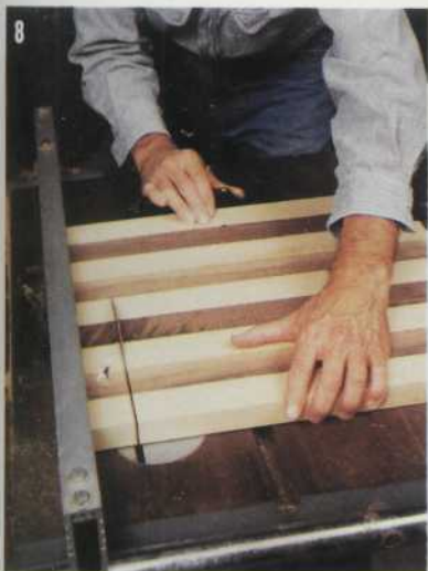
8 Reset the fence for a 1 3/4" cut and pass the board through the blade until you've got eight dark-and-light strips. Arrange them in the same order they've been cut.
