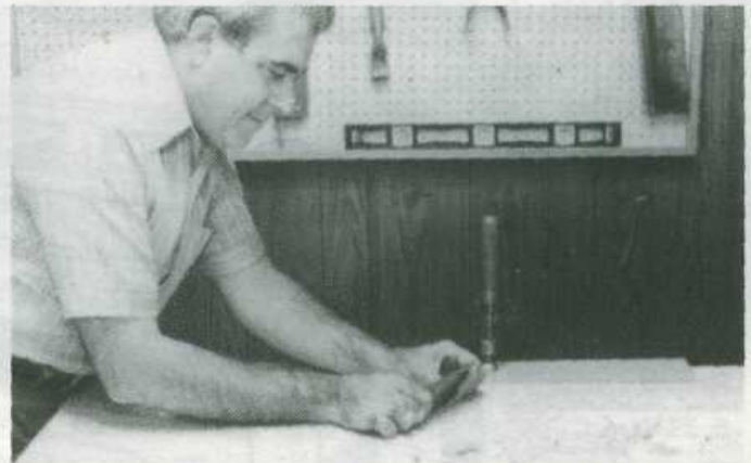
Fig. 23-4. Scrape glued board to make surface become smooth and even.
