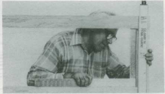
Fig. 24-2. Once the frame pieces have been cut, apply glue, insert the splines and clamp. Check to see if all right angles are true.
