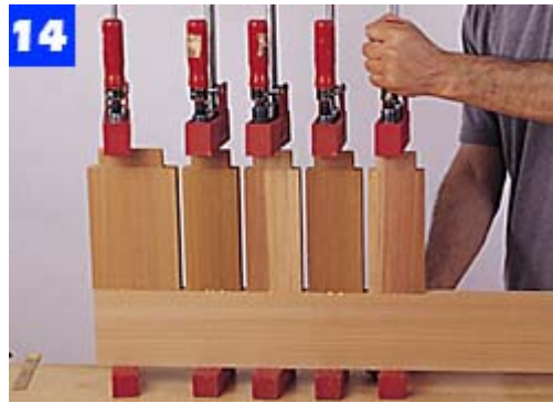
The first stage in assembling a benchtop is to glue and clamp slats to one stile. Use one clamp in the center of each slat.
