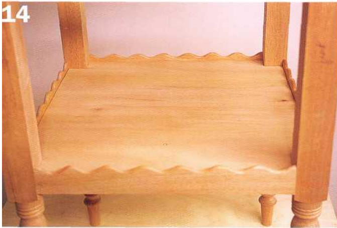
step 14 Make the cuts on the shelf and check the fit.
