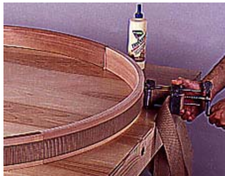
7 Transfer the cradle to a bench, and use it to hold the apron section in place while cutting the biscuit slots.
