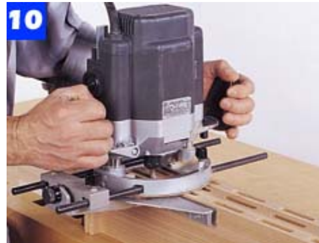
To cut the long row of mortises in each stile and rail, clamp three of the work-pieces together to support the router.
