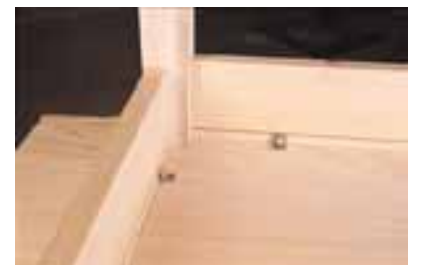
These table top fasteners are cheap ($1.99 for a pack of eight) and sturdy. Simply place the clip end into the kerf in your apron and screw the other end to your table top.
