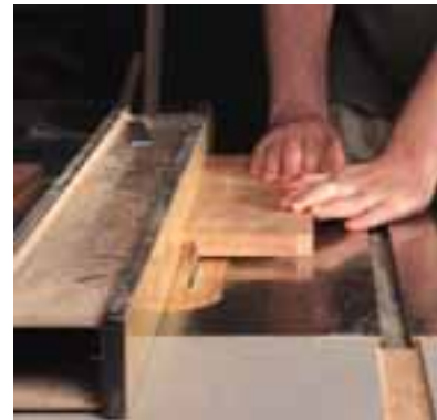
You will need to fasten the tabletop using tabletop fasteners, which requires making a kerf in the aprons. I made this kerf on the table saw 7/16" from the edge and ¼" deep.
