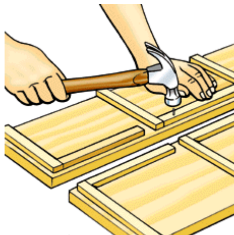
Fig. 5 Butt sides together with shelf-location marks on outer edges. Use a straightedge to extend the shelf marks across work.
