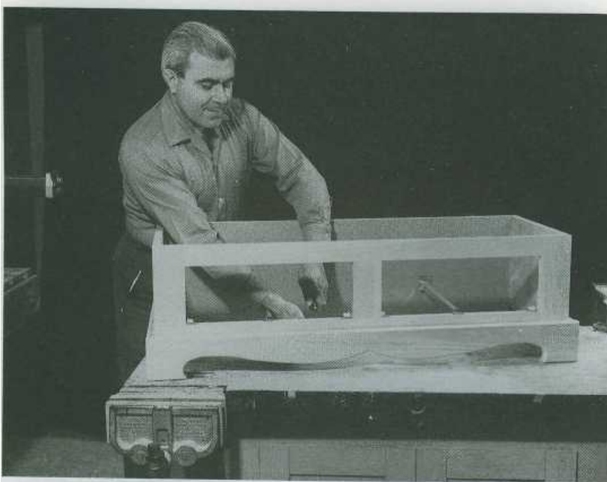
Fig. 9-5. The base section is fastened to the main section with the aid of screws. Note the single track drawer slide hardware. Knap-Vogt No. 1175 was selected for use in this project.
