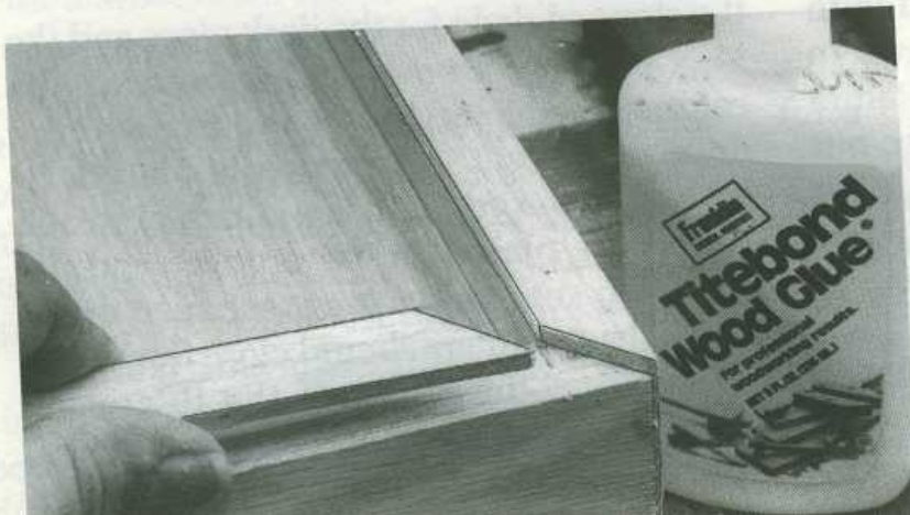
Fig. 25-10. Ends of the strips are mitered and each piece is carefully fitted. Apply glue to the plywood edge and strip and fasten with brads. See text regarding edging brads.
