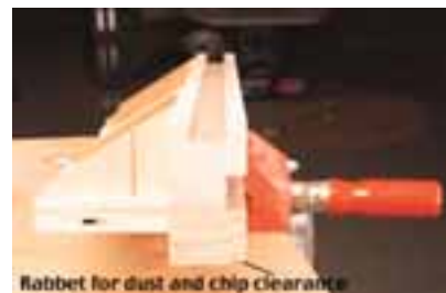
ROCK SOLID The fence is made of a sturdy, stable hardwood. Cut a groove the length of the top and face of the fence. The grooves support T-slot tracks, which can be used for stops, hold-downs and other accessories.
