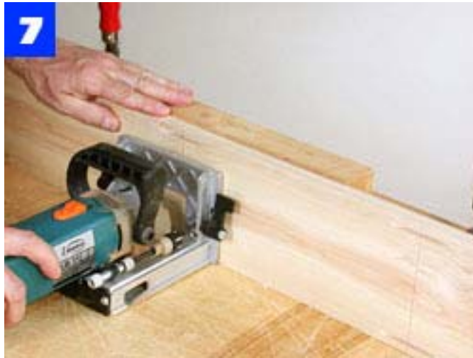
Lay out plate joints in the post parts and cut the slots. The plates keep the pieces aligned during assembly.
