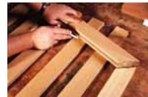
With the miters cut on the top rail and back stiles, space the slats and use the top rail to mark the angle and length of each slat, (adding 1").
