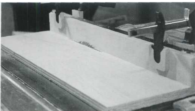
Shown here is the combination fence and throat I use for ripping inlay and cock bead.
