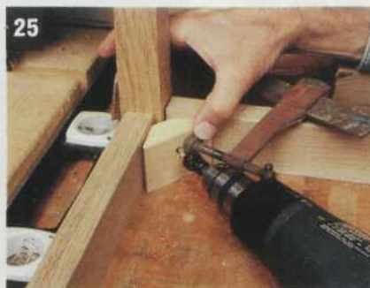
25 Set up the table frame on a flat work surface with a band clamp placed snugly around the frame's circumference. Use a #6 screw bit with the stop collar set at 1¾" to pre-drill a hole through each brace and then into the leg behind it. Center the hole ¾" from the exposed edge, and set the braces flush against the work table.
