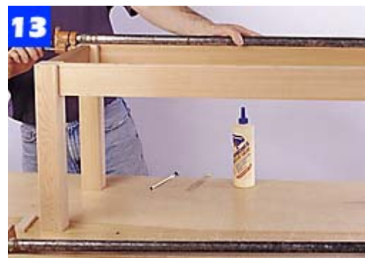
Join two leg-apron subassemblies spanned by a long pair of aprons. Glue and clamp this to complete a bench base.
