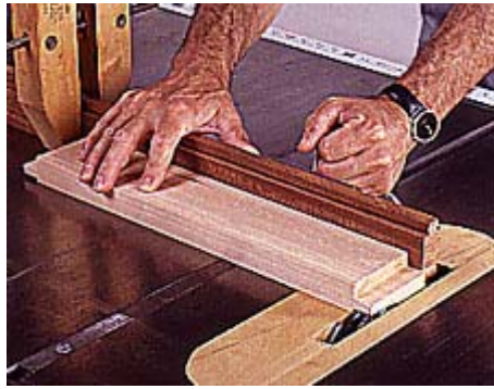
16 Clamp a stop to the miter gauge fence. Use a dado blade to cut the tenons on the rails, stretchers and back slats.
