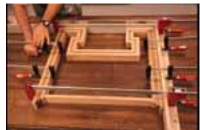
When assembling the legs to the Greek key, I used a spacer (seen at the bottom of the photo above) to keep the legs spaced properly while gluing-up.
