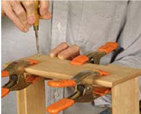
The top is screwed straight into the sides, then plugged and trimmed flush.
