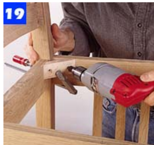
Join the back subassembly to the front-leg/side-rail assembly. Work on a flat surface so the legs remain even.
