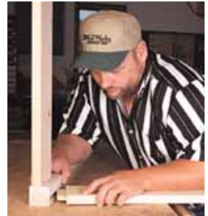
I usually build my tables using straight mortise-and-tenon joinery. However, there are special cases when other methods are just as good or even better.
