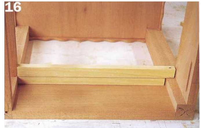
Step 15 Prepare the drawer runners and guides and make the tenon on one end of each runner. Remove the tenon at the front leg and cut a notch at the rear leg.
