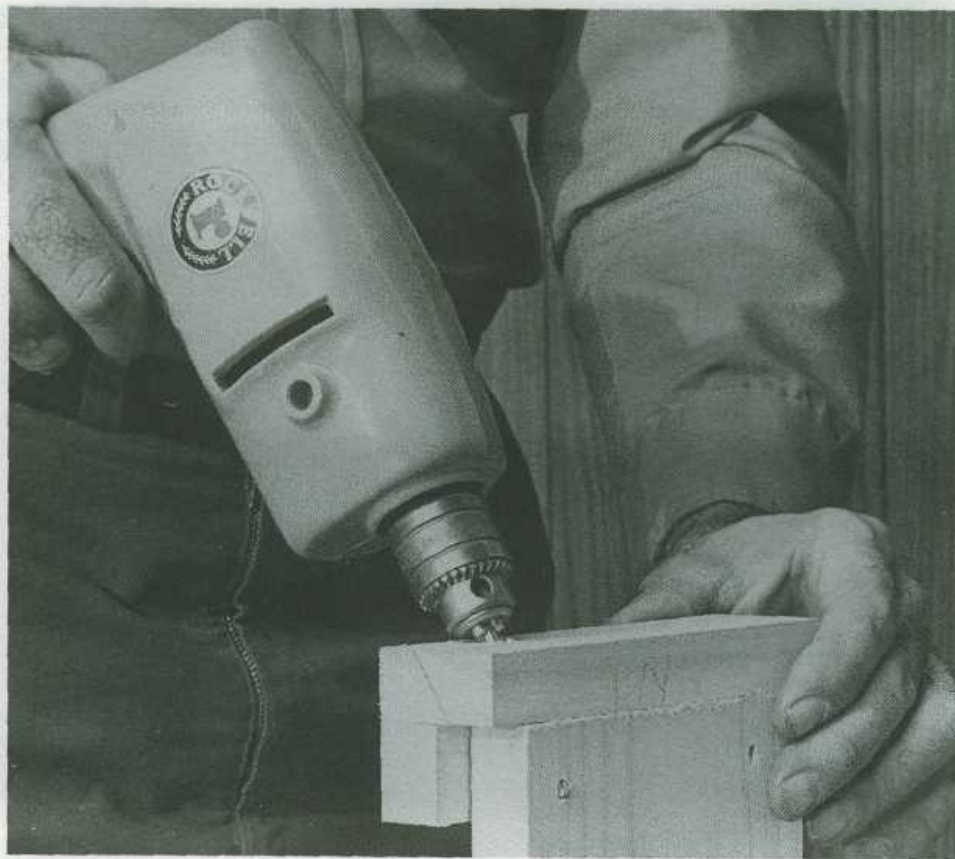
Fig. 8-14. A simple jig is used to drill the diagonal pilot holes for the screws. Make it from available scrap wood.
