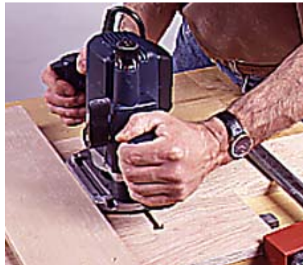
13--Rout slots in the drawer face for the drawer sides with a dovetail bit. Use a square U-shaped jig to guide the router.
