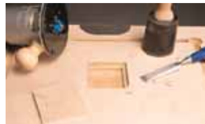
RABBET FOR THE INSERT After cutting the hole with a jigsaw, the opening is rabbeted using a bearing-piloted router bit. Then chisel the corners square and fit the replaceable center tightly into the rabbet. Make a couple extras.
