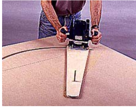
1 Make the bending form template with a plunge router on a trammel arm. Cut an arc in a sheet of MDF.
